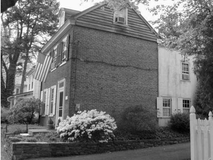
Illustration 30: Appropriate rear addition for its change of materials to stucco and location of addition at the rear
