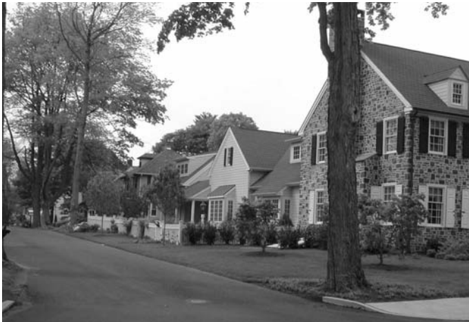
Illustration 42: Appropriate infill due to the continuity of the street wall, diversity of wall materials and consistency of fence and landscaping
